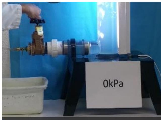
Figure 11: Result with bubble ingress
