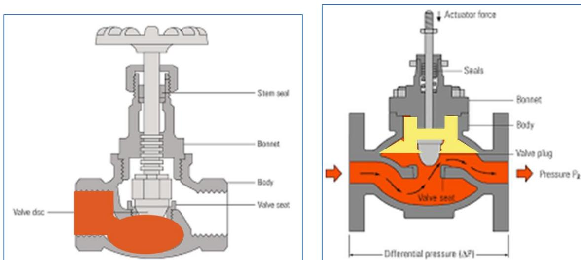
Figure 8: Minimal Danger with Globe Valve used as a transformer drain valve
