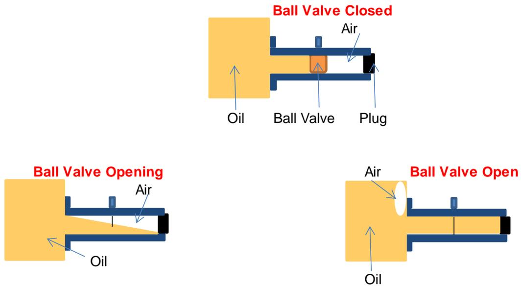
Figure 6: Danger of a Ball Valve when used as a transformer drain valve
