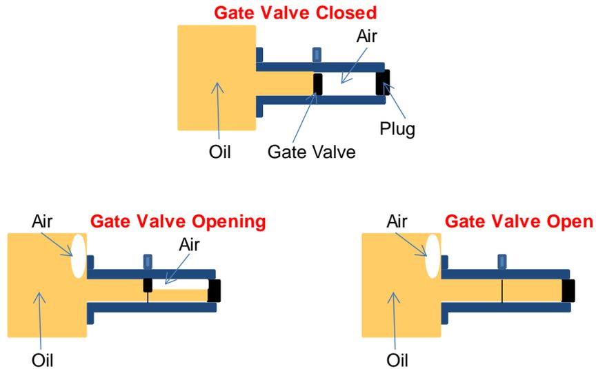
Figure 7: Danger of Gate Valve used as a transformer drain valve
